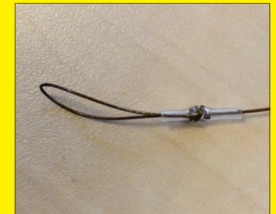
7. Finish it off neatly by placing a piece of shrink tube over the knot.
