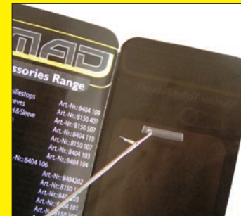
7. The most vital step for this rig; make a tiny hole in the tube with your needle just before the end
